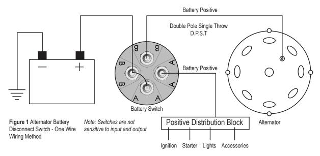
Good for two high current loads, 125A continuous, 750A intermittent (15 Seconds on, 5 minutes off), up to 36VDC Max. Both Poles are separately insulated. Operating Temperature Range is -40°F to 185°F (-40°C to 85°C). Studs use 3/8"-24 nuts (included).
