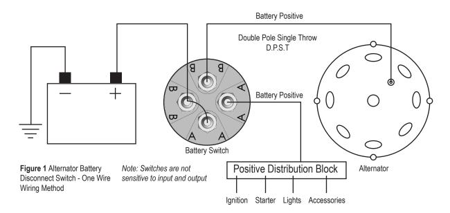
Good for two high current loads, 125A continuous, 750A intermittent (15 Seconds on, 5 minutes off), up to 36VDC Max. Both Poles are separately insulated. Operating Temperature Range is -40°F to 185°F (-40°C to 85°C). Studs use 3/8"-24 nuts (included).
